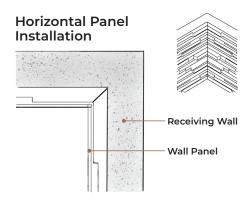
A seamless, inside corner can be achieved by joining panels using a miter joint.
