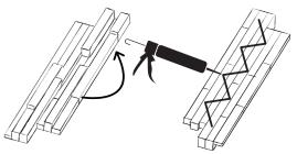
elastic MS polymer adhesive. As a guide, you will need one standard 10 fl. oz. tube of adhesive per 20 sq. ft. of paneling.
