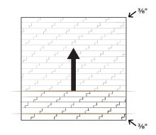
Continue to work bottom to top, left to right, as you add rows. After the installation of the first five rows, check that straight lines have been maintained, correcting if necessary.
