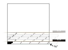
Position the first panels in a straight row on the wall. Remember to leave a 3/8" gap for expansion at the bottom of the wall.
